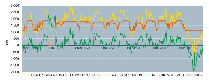
III. UNPLANNED OUTAGES: One: Tripped on 3/27 because of knock sensor required shutdown. Downtime
